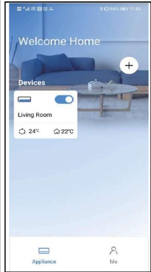
3. Thus, user can control air conditioners on/off status, operation mode, temperature, fan speed and so on.
